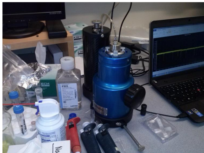
The qNano instrument for measurement of exosome concentration and size distribution
