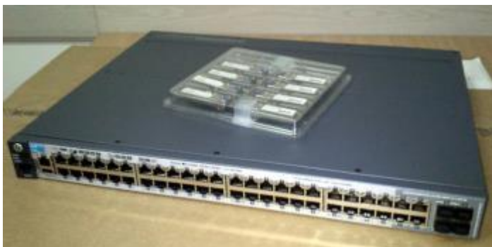
Photo 5: One of the four purchased LAN switches; the plastic transparent box on the top contains optical fiber communication modules.
