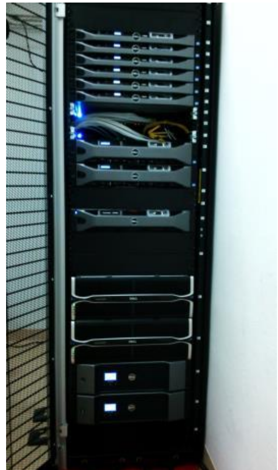
Photo 2 (right): The internals of the cabinet of the computing cluster: six computing servers at the top and mass storage devices in the lower part.
