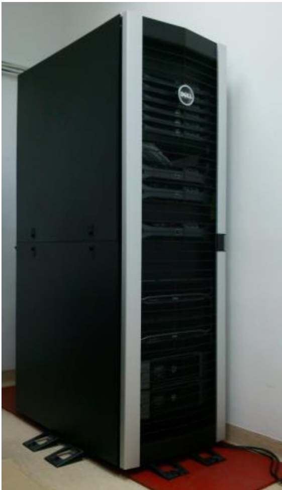
Photo 1 (left): The Rack cabinet containing elements of the computing cluster, namely mass storage devices and computing servers. This hardware is located in the server room of Department of Medical Genetics, MUW.
