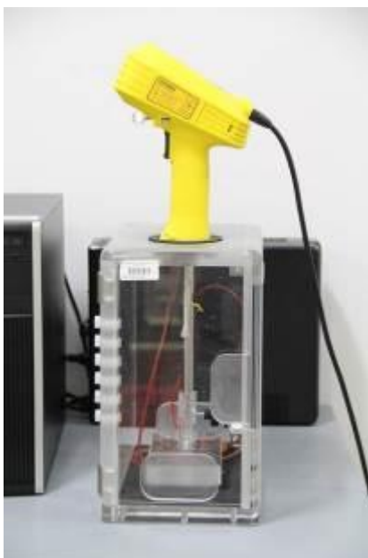
Photo 5: Hielscher Ultrasonics UP200ht handheld ultrasonic homogenizer installed in the Department of Immunology, MUW
