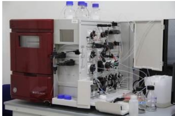
Photo 7: GE Healthcare preparative chromatography system AKTA avant 25 installed in the Department of Immunology, MUW
