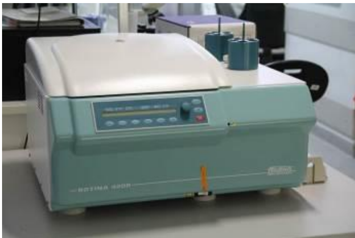
Photo 8: Andreas Hettich laboratory centrifuge ROTINA 420R installed in the Department of Immunology, MUW
