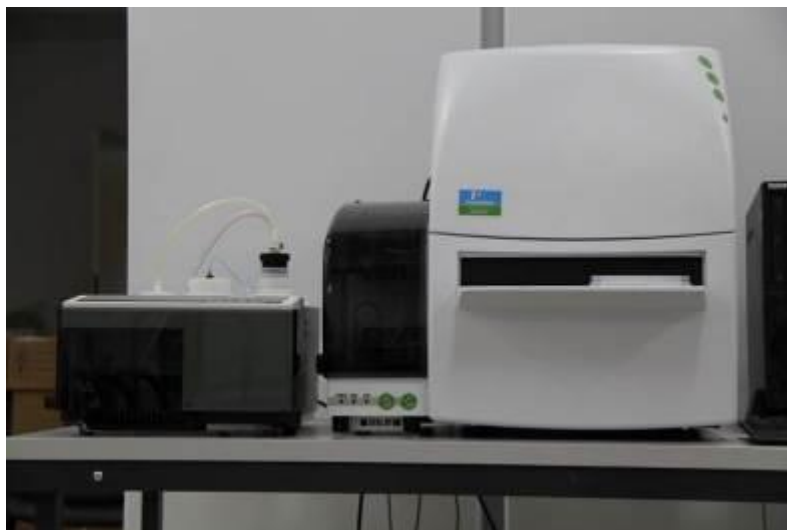
Photo 9: Delphia platewash and EnVision multilab plate reader installed in the Department of Immunology, MUW
